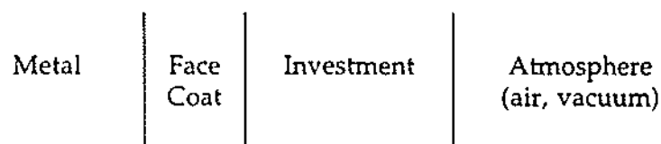
Figure 2 Schematic diagram showing the different thermal resistances involved in the heat transfer.
