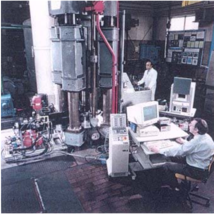
NPL's big friction rig is used to determine friction coefficients
