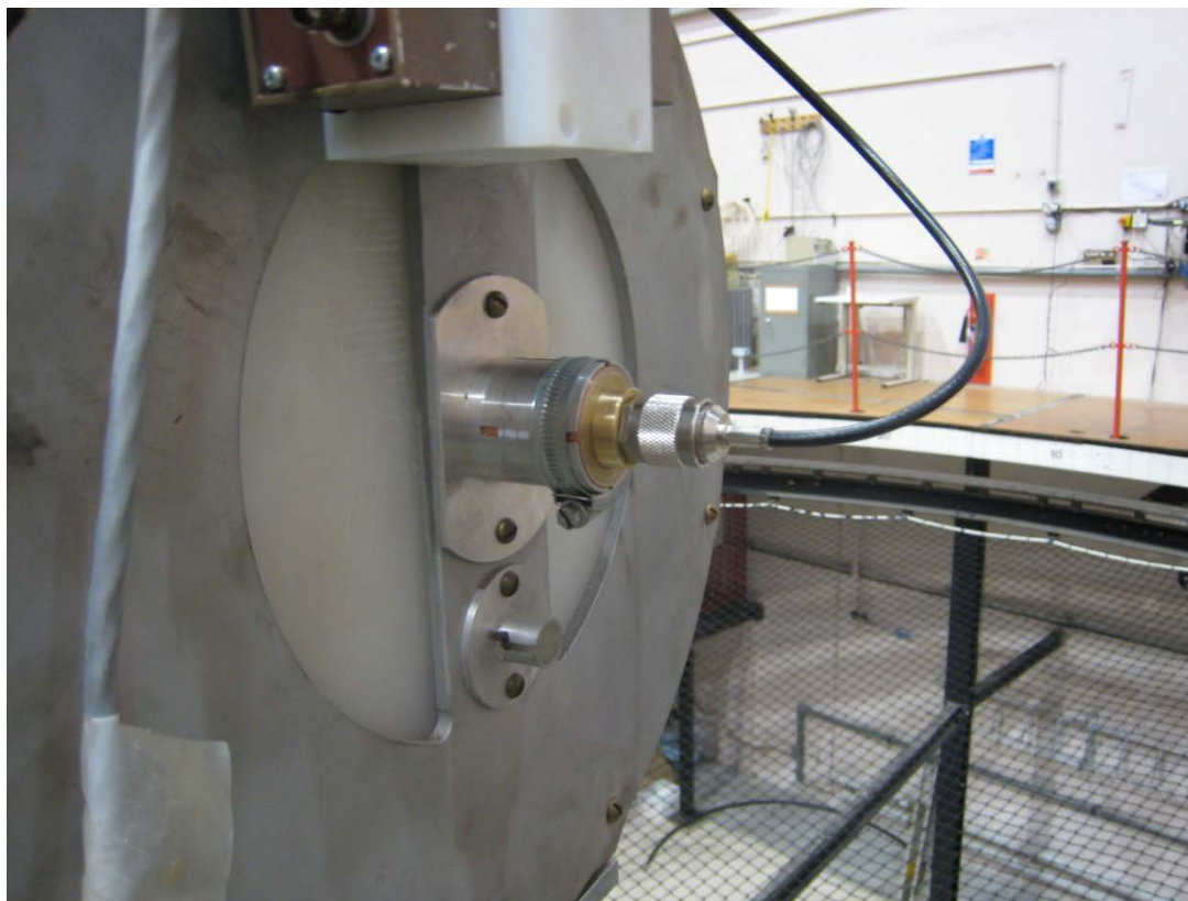
Figure 4. Positioning of the BF 3 counter in the long counter body.
