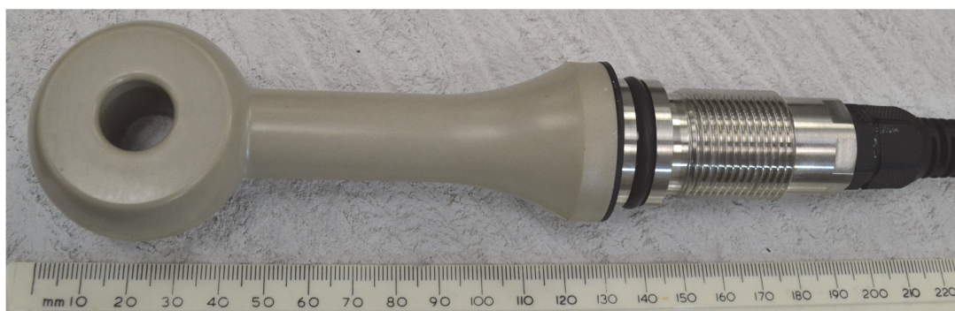
Figure 5: A commercial inductive probe (Mettler Toledo model InPro 7250 ST ) for measurement of static conductivity. All of the measurements of static conductivity presented in this report were made with this probe in conjunction with conductivity-meter model M400 Type 1 Cond. Ind. This system does not allow permittivity to be measured.
