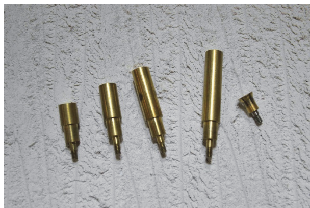
Figure 14: Truncated inner conductors (lengths 7, 12, 18 and 25 mm) that can screw in place of the spring-finger collet (shown right) of an MPC14/ GR900 coaxial-line connector. These are used for measurement on liquids and also as offset open-circuit standards for calibration.
