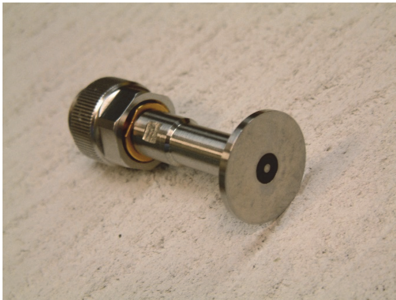
Figure 7: NPL Ø 7-mm coaxial sensor (frequency range 100 MHz to 10 GHz). The bore diameter is 7 mm and the flange diameter is 25 mm.
