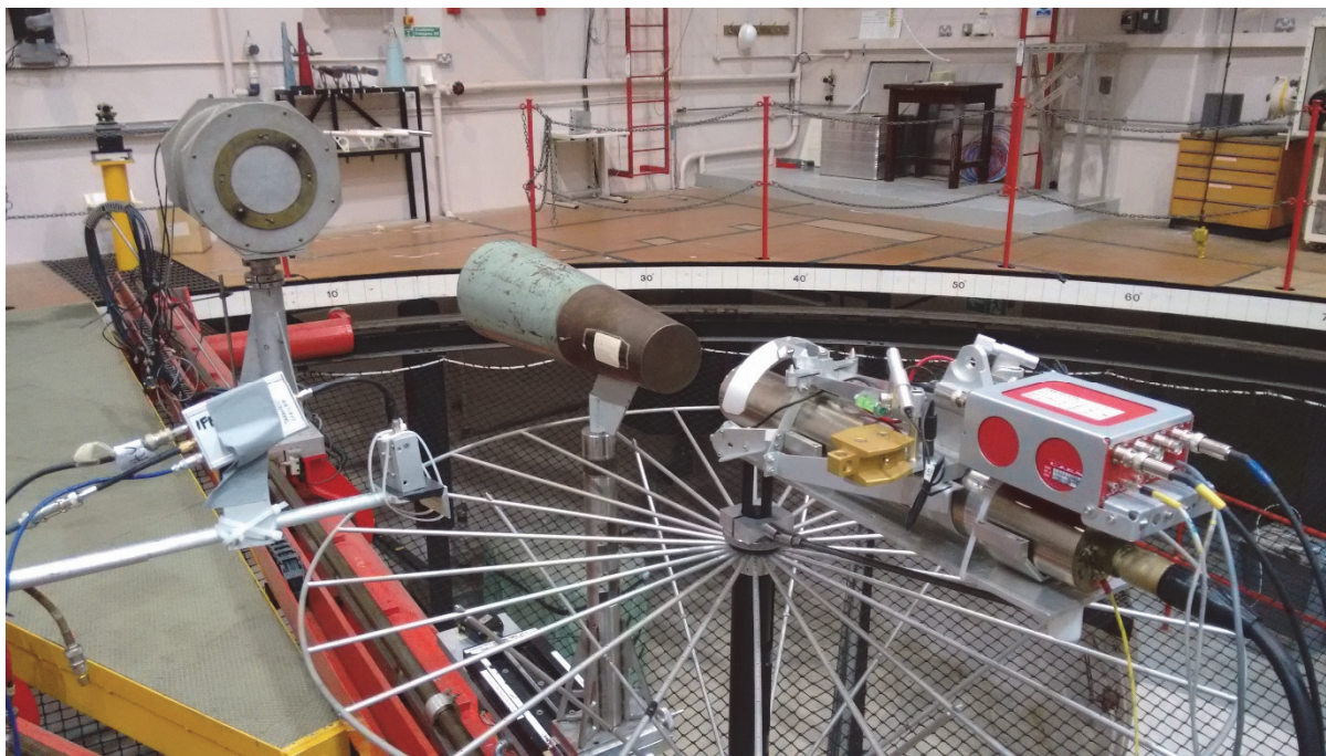
Figure 2. The De Pangher LC, top left in the picture, mounted in the NPL low-scatter area with the NG to the right and a shadow cone between these two devices. The device in the foreground to the left is a diamond detector. The target of the NG is positioned at the centre of the circle about which the LC was rotated.
