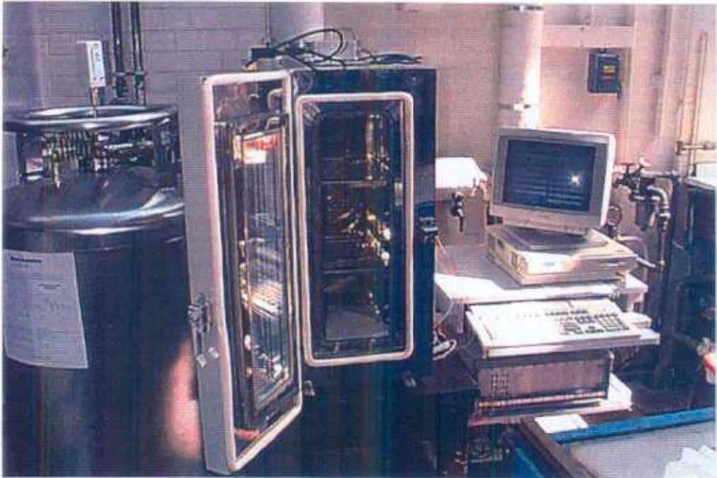
Figure 3: Thermal expansion equipment
