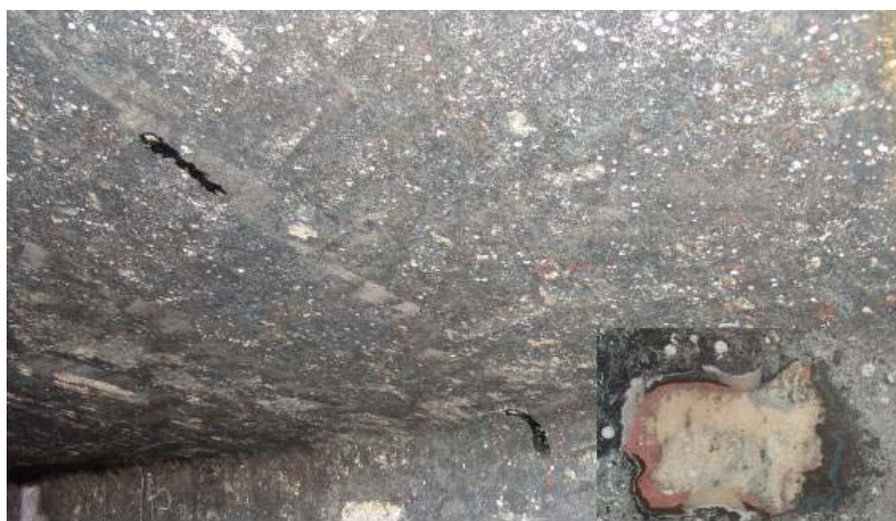
Figure 2.3 Osmotic blistering of a GFRP boat hull with inset showing laminate breakdown (Courtesy of Minton, Treharne and Davies Ltd)
