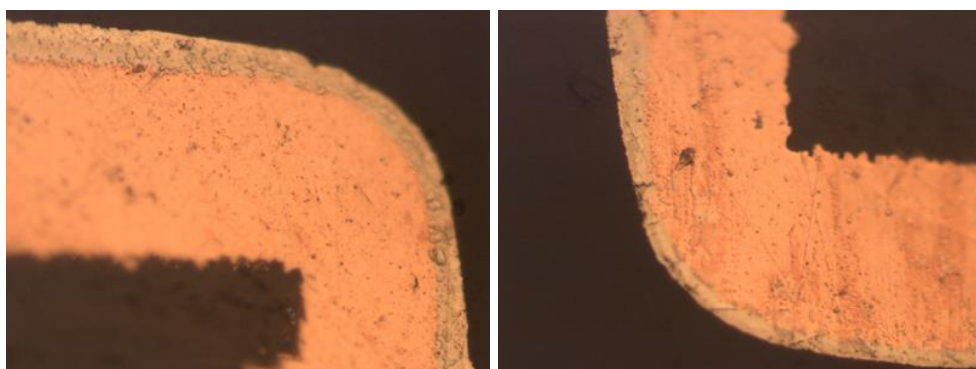
There was no evidence of cracking on the knee of plated through holes or at the through hole plating to inner layer junctions
