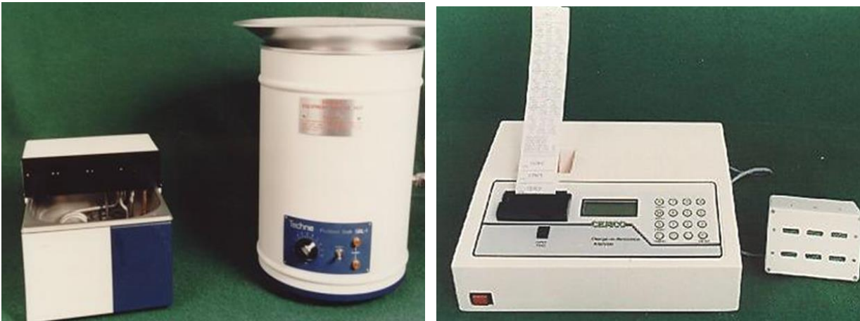
Images above show Cemco equipment used for thermal shock. On the left is the water bath and fluidised sand bath, on the right is sample head and measurement system
