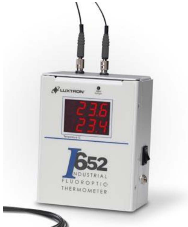
Figure 1: The Luxtron I652 two-channel fluoro-optic thermometer, which claims a “0.2 °C accuracy”.
