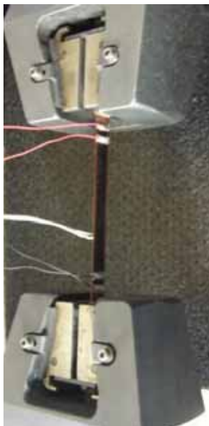
Figure 30: Unidirectional GFRP tensile specimen with a CNT/epoxy coating
