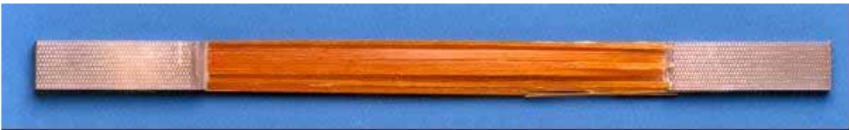
Figure 51: Longitudinal splitting in fatigued unidirectional GFRP
