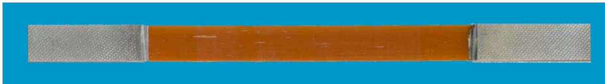
Figure 50: Fibre debonding and matrix cracking in fatigued unidirectional GFRP (damage indicated by narrow, whitened areas along gauge-length)
