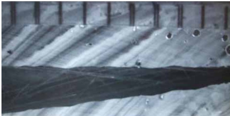
Figure 41: Optical image of mode I crack with extensive fibre bridging
