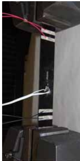
Figure 35: Four point method for measuring surface resistance of CFRP in tension
