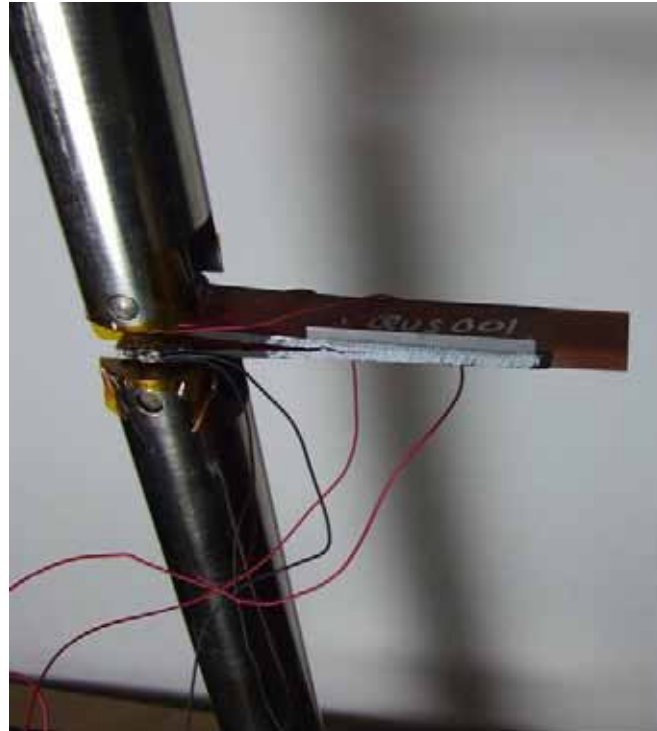
Figure 39: Mode I test of UD GFRP DCB specimen with a CNT/epoxy coating (Electrodes attached to specimen edges)
