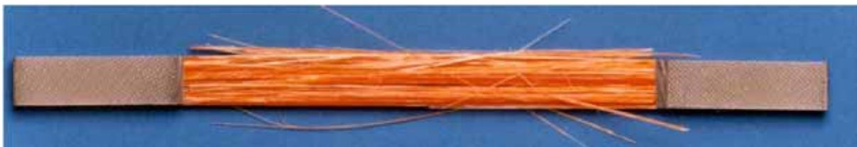
Figure 52: Typical tensile failure for monotonically loaded unidirectional GFRP
