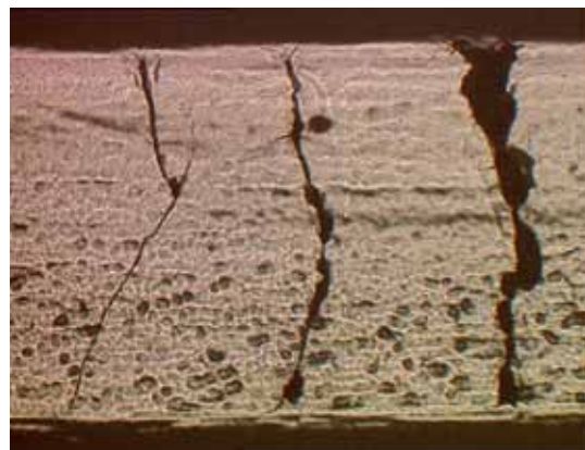
Figure 59: Transverse cracks along an edge of a cross-ply laminate
