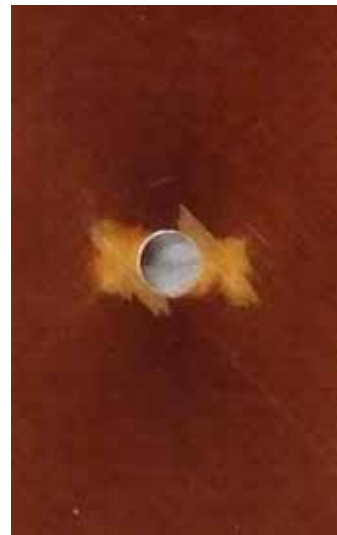
Figure 65: OHT test set-up showing damage around the hole
