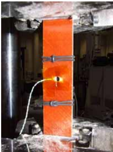
Figure 65: OHT test set-up showing damage around the hole
