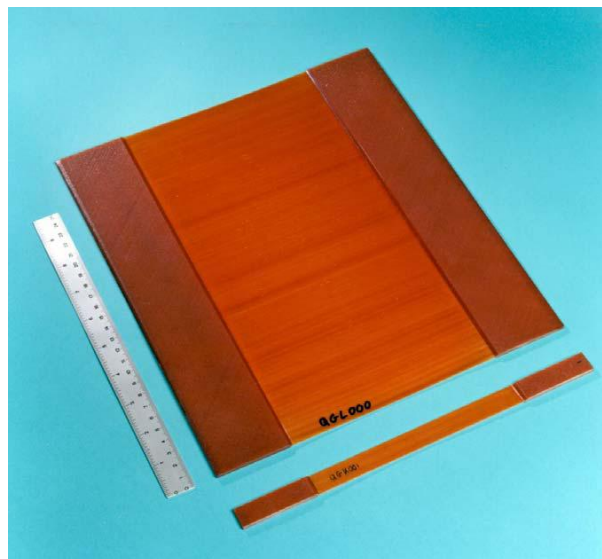
Figure 23: Unidirectional E-glass/epoxy laminate with bonded end tabs
