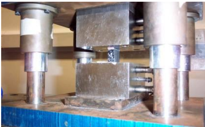
Figure 51: End-loading compression fixture with specimen
