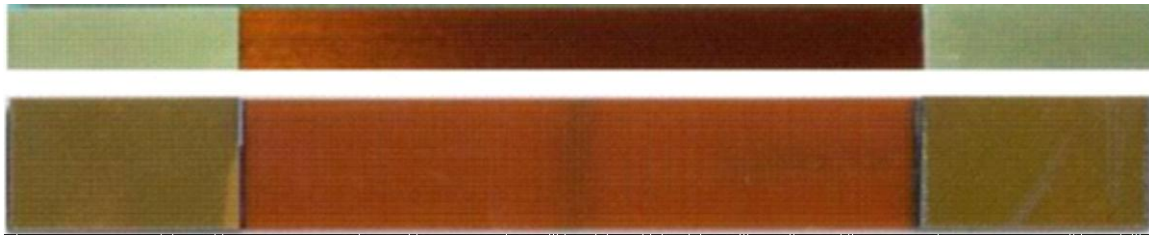
Figure 22: Longitudinal (top) and transverse (bottom) tensile specimens
