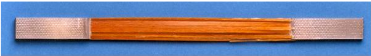
Figure 28: Longitudinal splitting in fatigued unidirectional GFRP
