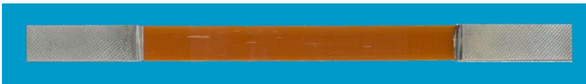
Figure 27: Fibre debonding and matrix cracking in fatigued unidirectional GFRP (damage indicated by narrow, whitened areas along gauge-length)
