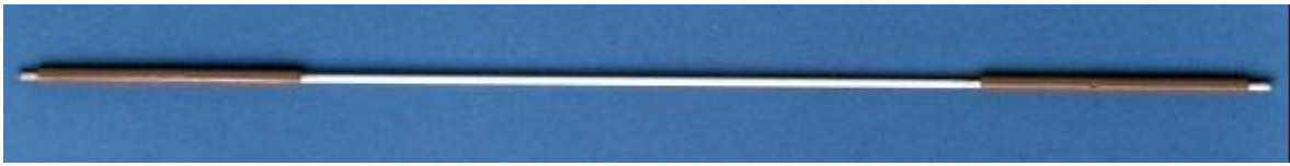
Figure 19: Composite rod specimen with moulded end tabs
