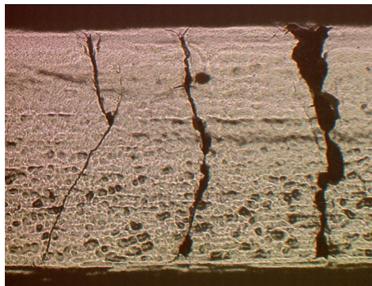
Figure 36: Transverse cracks along an edge of a cross-ply laminate
