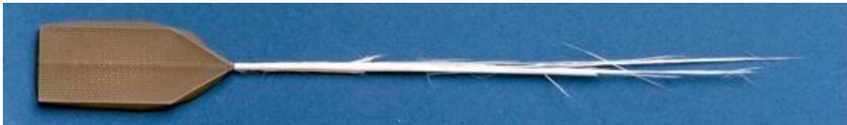
Figure 20: Typical cyclic fatigue failure for glass/polyester rod specimen
