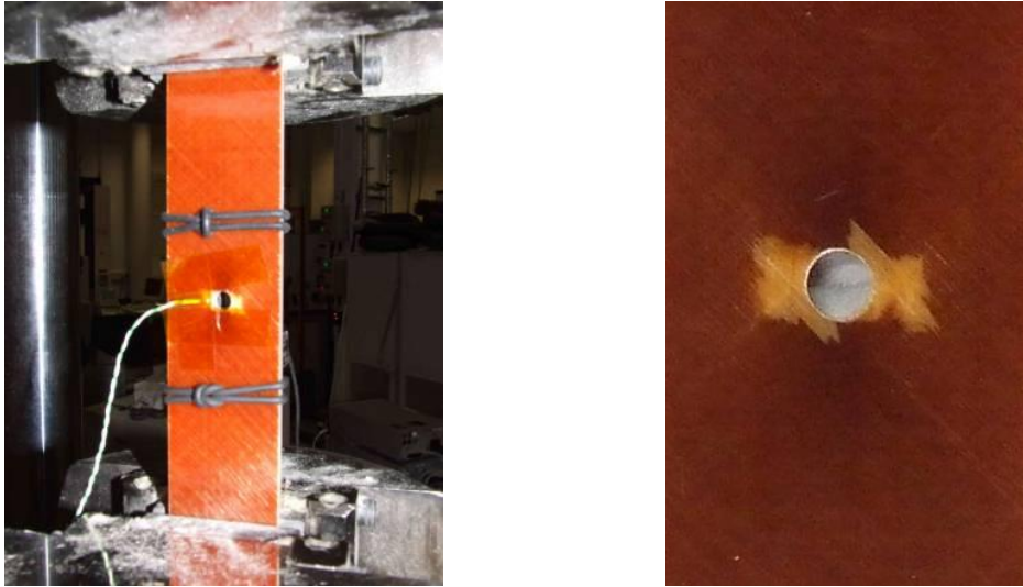
Figure 44: OHT test set-up showing damage around the hole
