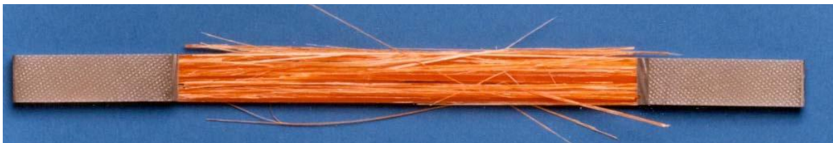
Figure 29: Typical tensile failure for monotonically loaded unidirectional GFRP
