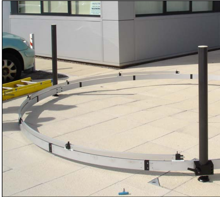
Figure 11: The arm-mount runners are mounted on the base-ring
