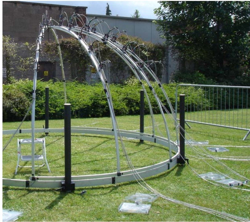
Figure 18: The optical fibres should be fastened to the structure to avoid any bends that could damage them
