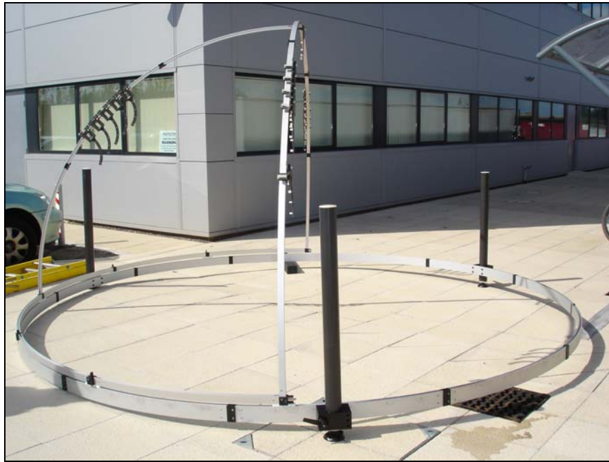
Figure 2: The next phase involved constructing the arms. Arms 1 and 7 are built first, to form an arch using the nadir joiner. Arm 4 is then added to stabilise the structure.
