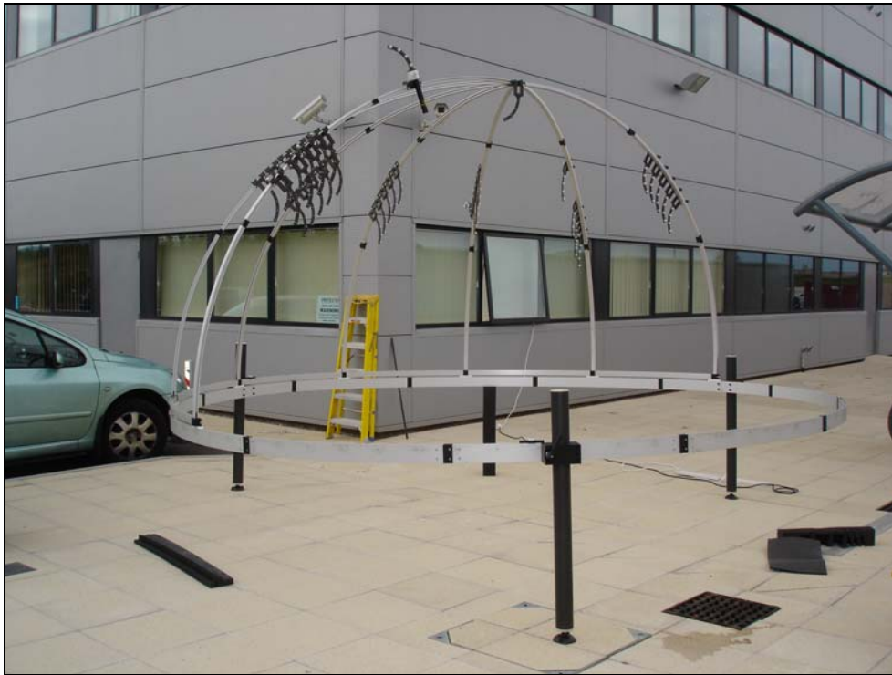
Figure 4: If required the structure can be been raised on its legs so that it is about 1m off the ground.
