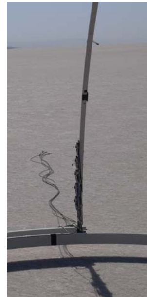
Figure 14: The optical fibers should be kept in the protection box before coupling them to multiplexers
