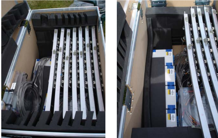
Figure 12: The Cameras and the Optical fibers are on the bottom sections of the arm runners
