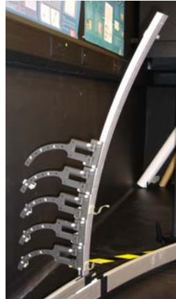
Figure 13: The bottom arm runner are attached to the base-ring
