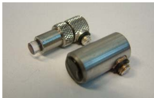
Figure 19 30MHz transducers: polystyrene delay line (left) and silica delay line (right)
