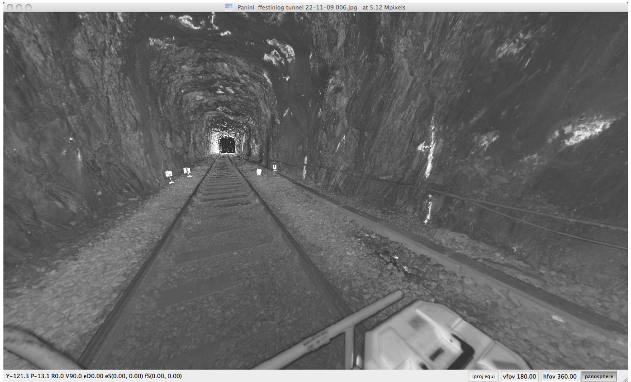
Figure 17. An equi-rectangular panorama produced by ScanTech and rendered using Panini, showing a forward view of the Ffestiniog Tunnel. The targets used for aligning each stationary scan can be clearly seen.
