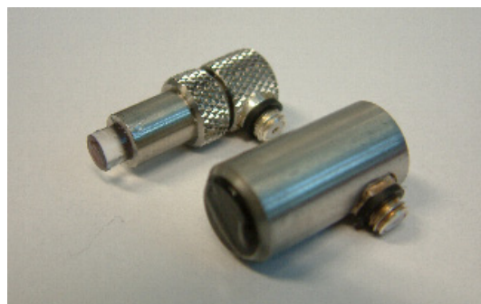
Figure 3 30MHz transducers: polystyrene delay line (left) and silica delay line (right).
