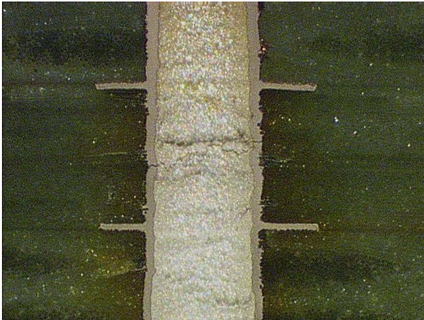
Figure 8: Micro-section of via with failure in region where non-functional pads have been retained.
