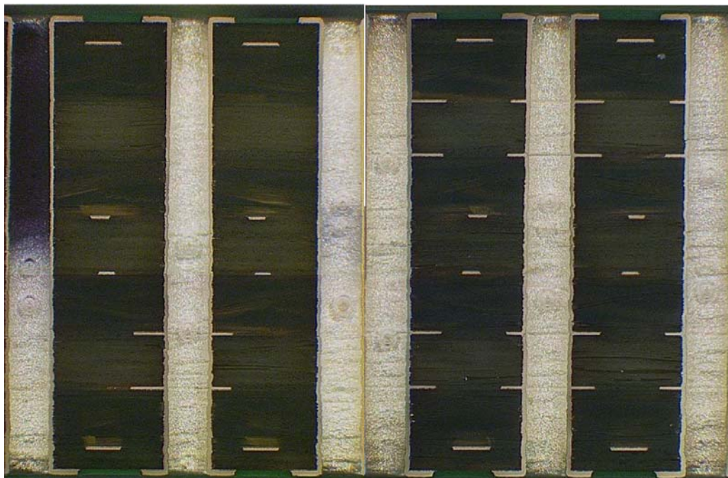
Figure 4: Micro-sections of thermally cycled vias showing non-functional pads excluded (left) and included (right)
