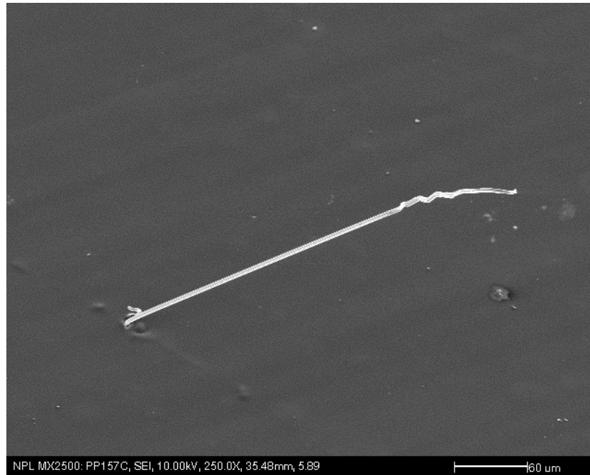
Figure 18: Typical erupting whisker (~300 \mu\text{m} in length) on acrylic sample.
