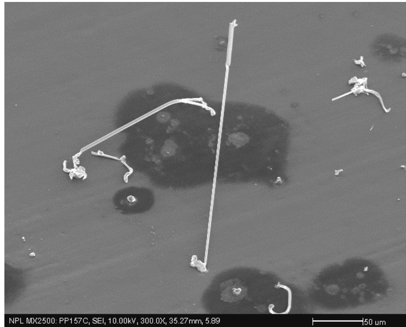
Figure 16: Typical erupting whisker (~250 μm in length) on acrylic sample.
