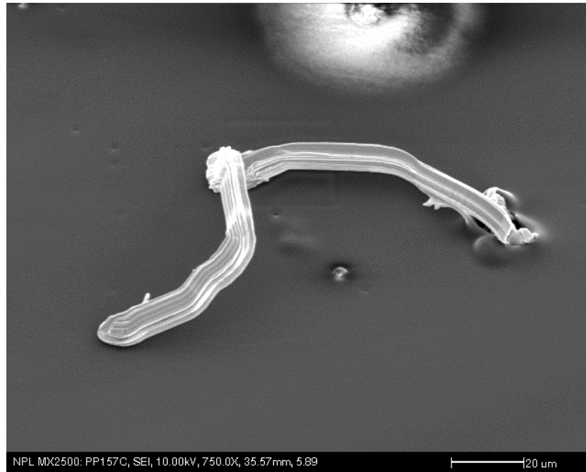
Figure 14: Typical erupting whisker (~150 μm in length) on acrylic sample.
