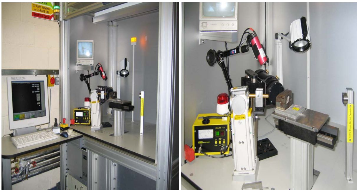
Figure 4.2: Example side-reflection real-time system.
