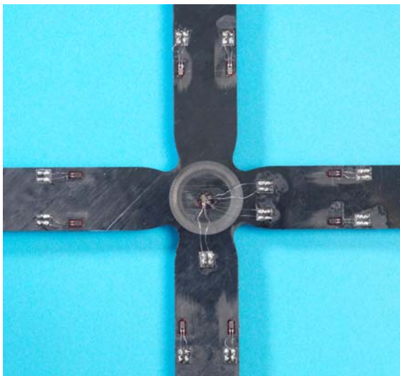
Figure 8: Arm and gauge-section strain gauges on a 25 mm specimen
