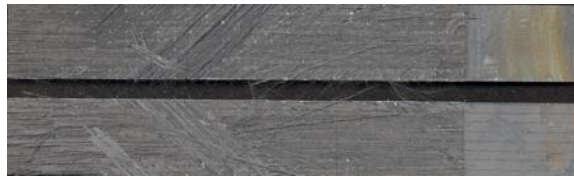
Crack in 0° ply
