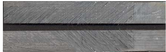
Crack in ±45° ply
