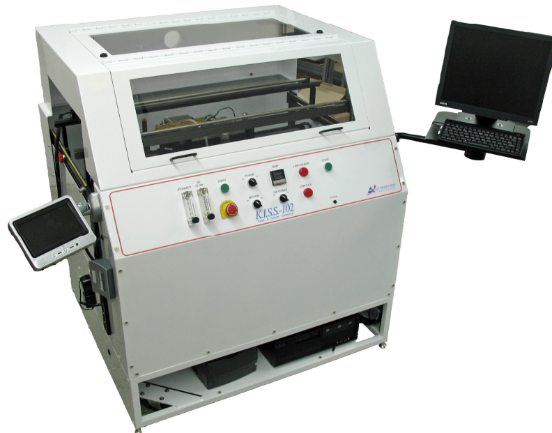
Figure 3: ACE soldering machine used for copper dissolution tests.
