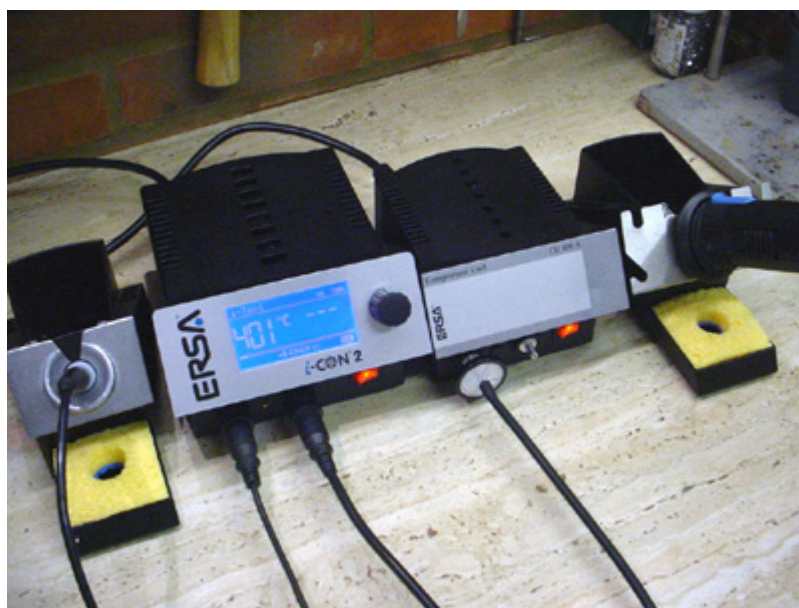
Figure 35: Photograph of the manual soldering tools used during trials
