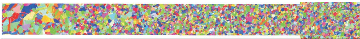
Figure B22 EBSD map of grain orientation in a section taken from a uniaxially compressed sample of 316L stainless steel. Top surface on left of map, centre of sample on right.
