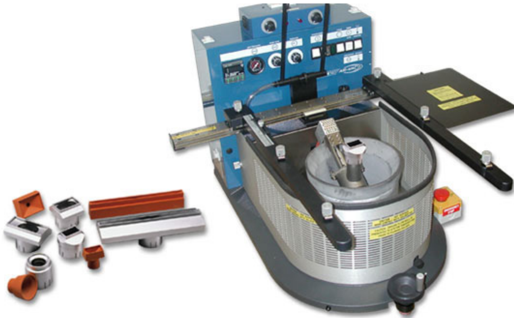
Figure 8 Typical solder fountain equipment. (Example image kindly provided by ZEVA)
