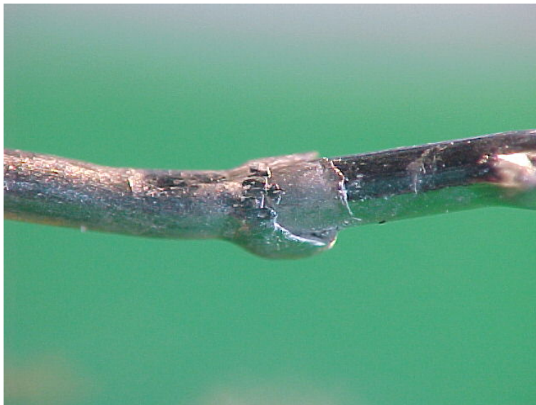
Figure 20: Copper dissolution of copper barrier layer on steel pin. Lack of a barrier layer on the base material has prevented a true bond forming on the surface of the steel surface. Copper or nickel barrier layers are often used to provide ease of soldering
