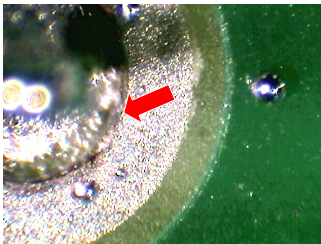
Figure 4: Loss of through hole connections where the knee/pad of the plated hole has been dissolved during selective soldering with a lead-free alloy. The surface pad finish on this board was copper Organic Solderable Preservative OSP.
