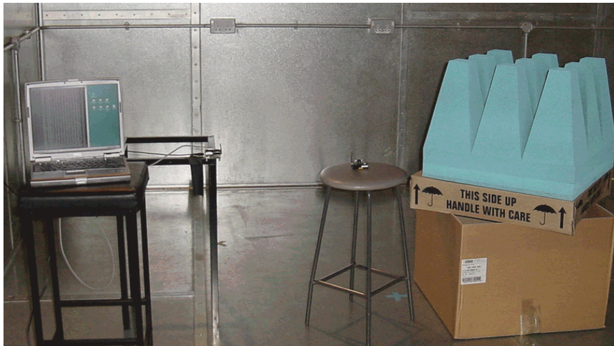
(b) Chamber with RAM and roughly placed node/base station
