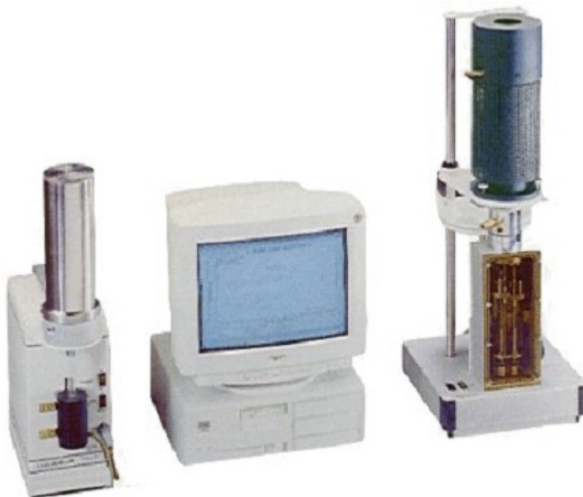
Figure 5: Dilatometer equipment used for measuring z-axis CTE
