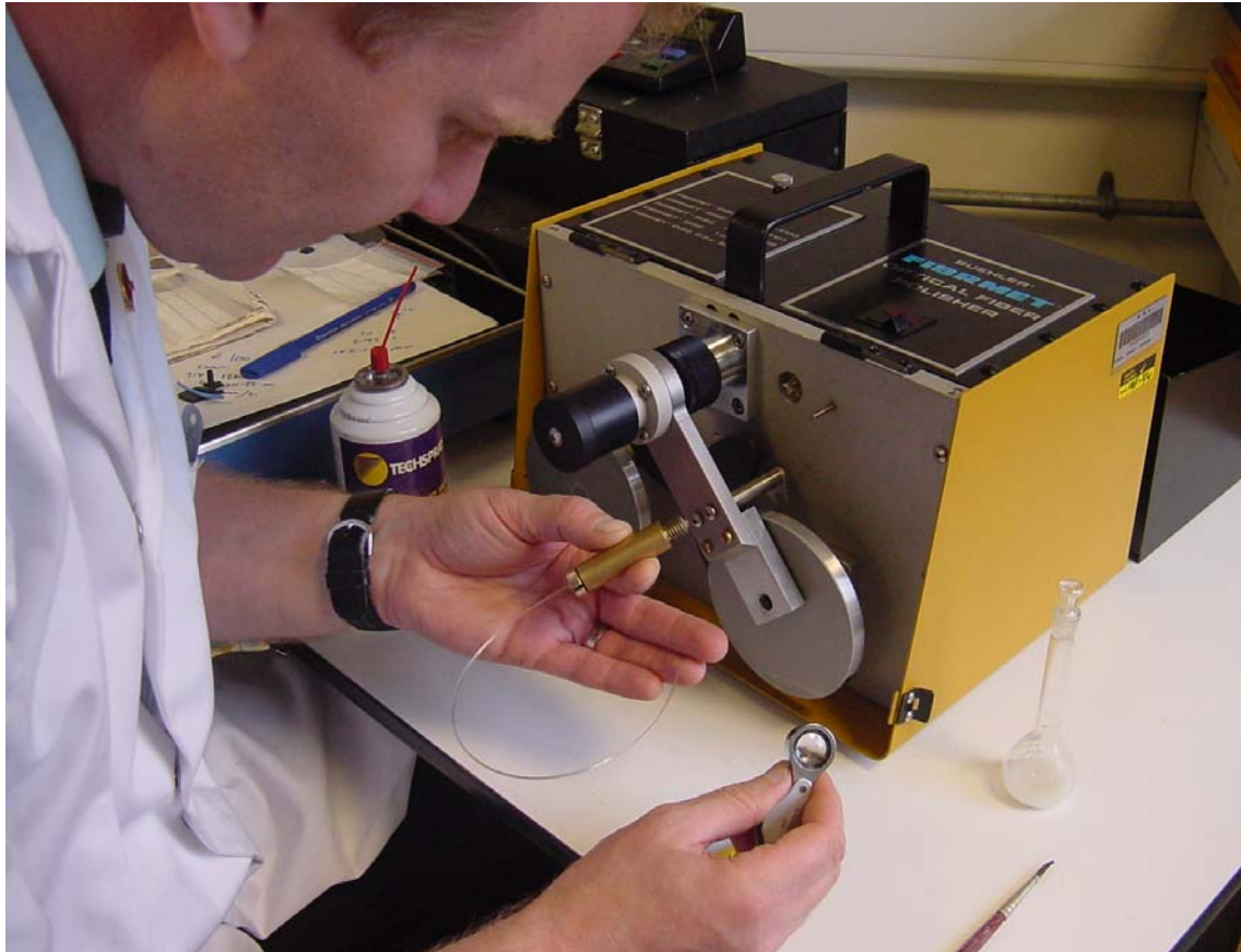
Figure 7 Machine tooling used for polishing POF
