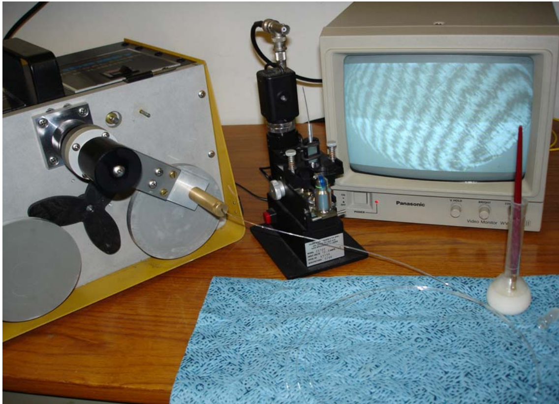
Figure 8 Photograph showing polishing machine tooling and interferogram of end face of a sample of POF using a 'Norland Microinterferometer'.
