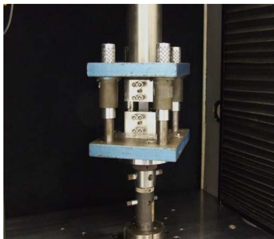
Figure 5 - End-loading compression jig mounted on hydraulic fatigue machine
