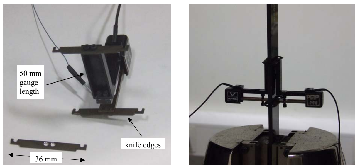
Figure 3.12: Extensometers used for measurement of strain in OHT tests
