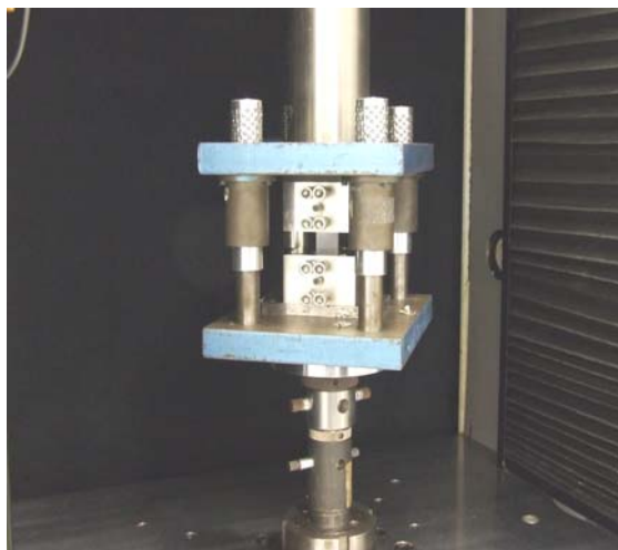
Figure 3.5: End-loading compression jig mounted on hydraulic fatigue machine
