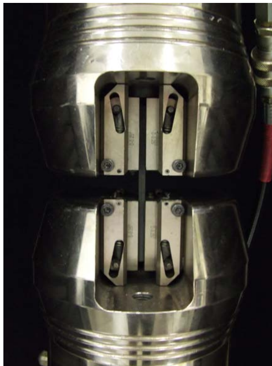
Figure 3.19: OHC specimen gripped in hydraulic wedge action grips
