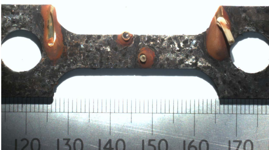
Figure 6. Photograph showing pitting in the SENT specimen after testing in aerated 1.5 ppm \text{Cl}^- solution at 90 °C for 2667 h.
