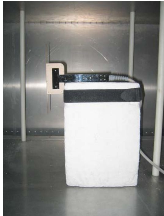
Figure 6. The robust sensor mid-way between the plates of the EMCO TEM cell. NPL uses this cell to calibrate field probes and loop antennas up to 60 MHz.
