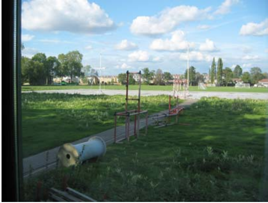
Figure 2. The NPL ground plane viewed from the measurement hut. There is approximately 50 m of low loss heliax cable underground, accessed by bulkhead connectors, one end shown in Fig. 3. The calculable dipole is connected to a further 15 m of coaxial cable. A 6 dB pad was used to reduce mismatch effects. The insertion loss of the cable run was measured using an additional 50 m of cable and the network analyser shown in Fig. 3. A biconical antenna was used, at a height of up to 5 m, to transmit the field.
