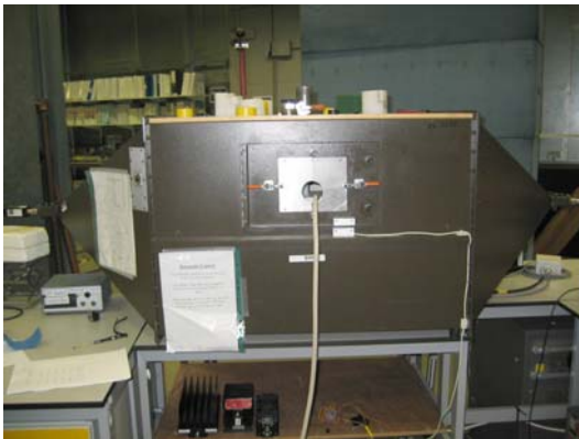
Figure 4. The IFI TEM cell
