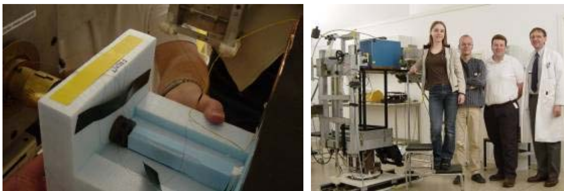
Figure 8. Left: calorimeter body, with part of its styrofoam surround. The final collimator of the proton beam line is visible at the left. Right: calorimeter housing (blue) in front of the proton beam line, with the team that performed the first ever therapy level absolute dose measurements using a graphite calorimeter in a clinical proton beam; from l. to r.: Mary Simon, Hugo Palmans, Russell Thomas (NPL) and Andrzej Kacperek (CCO)
