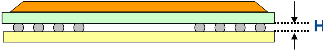
Figure 4. Gap between board and BGA component
