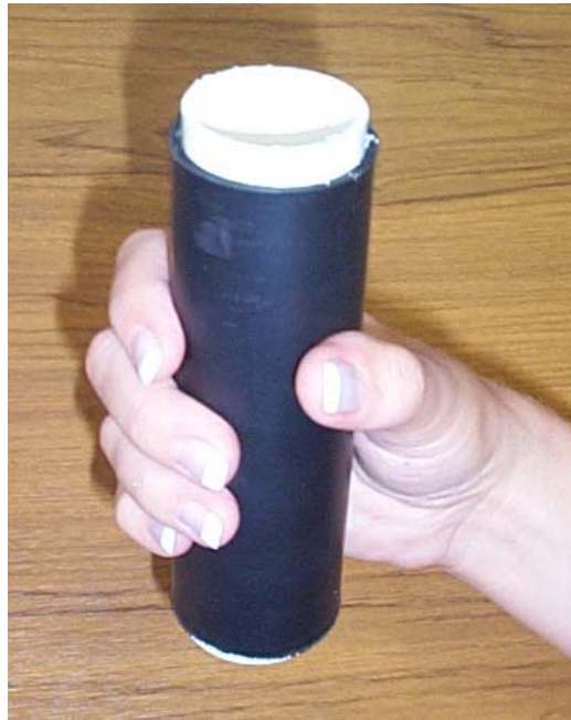
Figure 4: Procedure to assess the softness of a cylindrical sample
