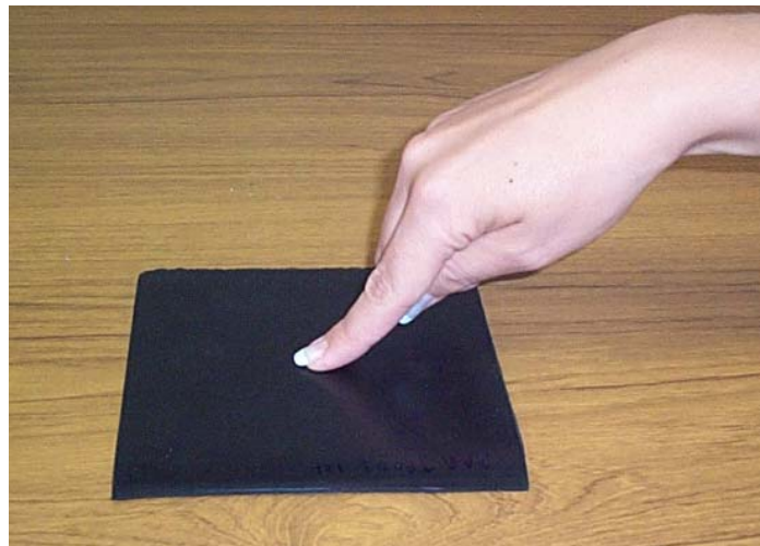
Figure 3: Procedure to assess the softness of a flat sample
