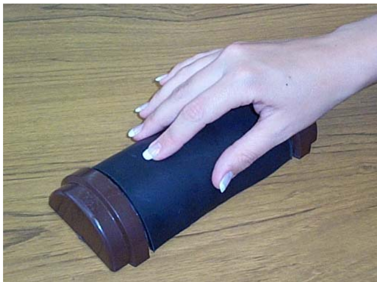
Figure 5: Procedure to assess the softness of a curved sample
