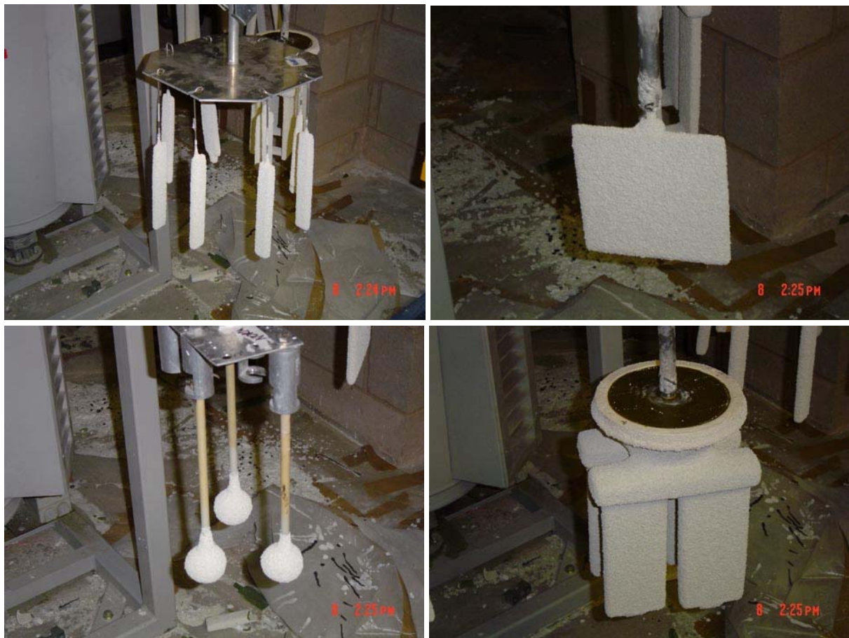
Figure 5: Dipped moulds, from top left clockwise: MOR bars, plates, bulge test moulds, permeability moulds.
