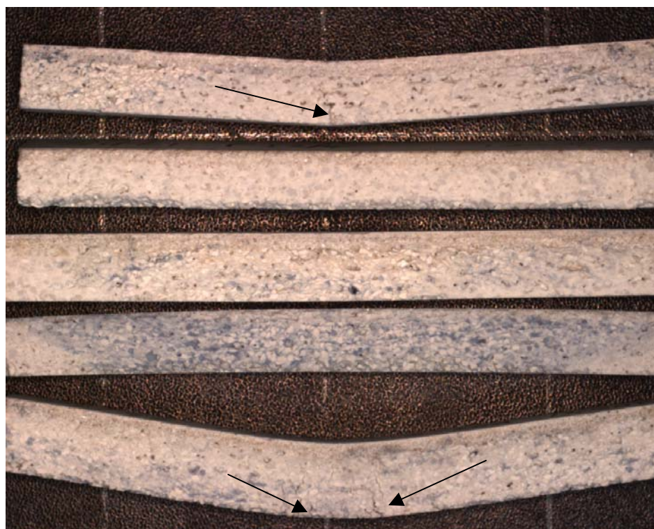
Figure 26: Flexural creep test-pieces of Partner 1, PJS, with test conditions shown at the right. The appearance of cracks is arrowed. Test 81 under no applied force shows reverse bending, while test 82 heated under load from cold shows much greater deformation than any other condition.
