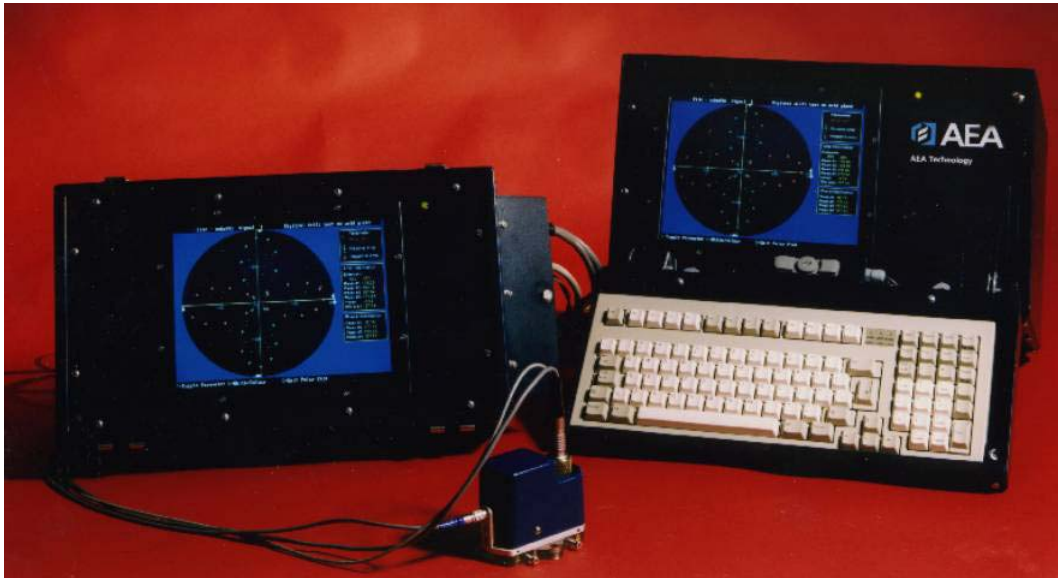
Figure 19. MAPS analogue biaxial stress system; showing PC, remote unit and motorised probe head.
