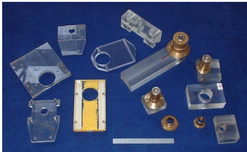
Figure 15. Examples of MAPS guide blocks (right) for manual probe rotation and face plates (left) for motorised measurement. These are shaped to match the geometry of the application.
