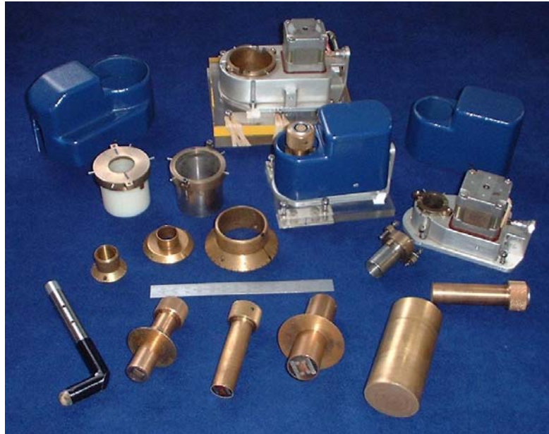
Figure 14. Examples of MAPS probes and motorised units of various sizes together with collars for assembly of the probe into a motor unit or for hand rotation using an angle calibrated guide block (not shown). Ruler length is 150 mm.
