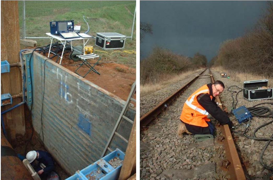
Figure 20. Examples where MAPS PC unit is remote from the probe unit using the umbilical.
