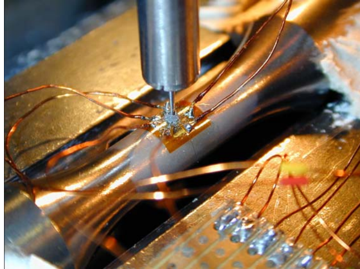
Figure 4. Hole drilling set-up
