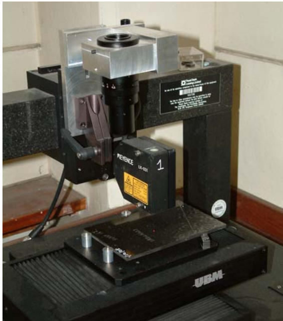
Figure 3 - Laser profilometer apparatus used for dent depth measurements
