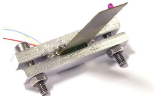
Figure 31 – Clamping arrangement for planar bimorph; 35 mm free length.
