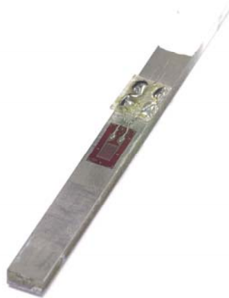
Figure 22 – Strain-gauged cantilever for system calibration.
