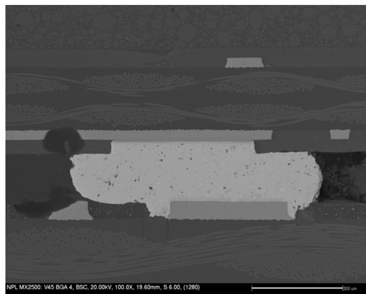
Figure 10. Section of Age 2 BGA component after manufacture
