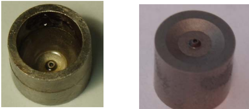
Figure 14: Short and long dies for separation of shear and extensional flow behaviours, and illustration of the nozzle geometry to avoid drooling of extrudate at the die exit.
