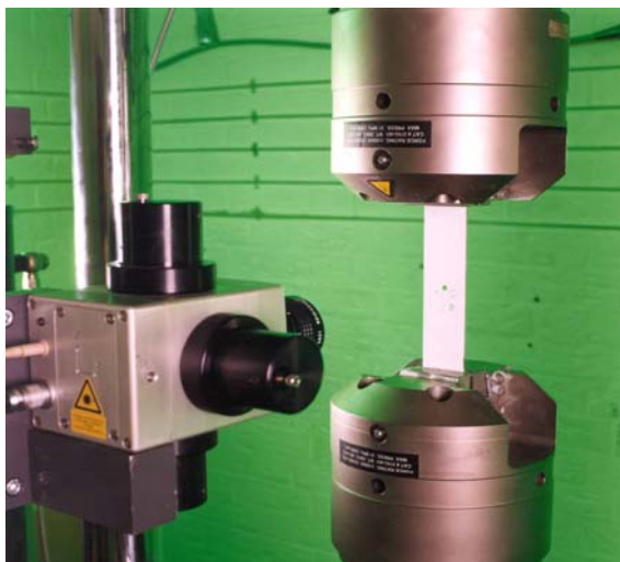
Figure 3 - Layout of the ESPI deformation measurement system
