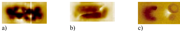
Figure 13. MFM images of NiFe rectangular particles with lateral dimensions 300×900 nm and thickness: a) 50 nm – multidomain (double diamond state); b) 30 nm – Landau state (a domain wall with width of 40 nm is clearly observed) and c) 10 nm – quasi single domain or ‘flower’ state.
