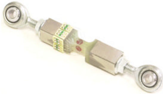
Figure 10 - Assembled miniature specimen with loading arms.
