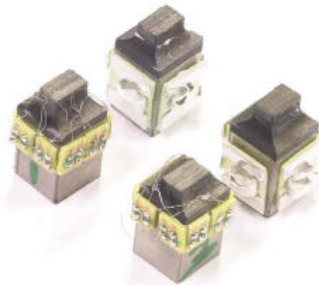
Figure 11 - Typical Type C specimen failures.
