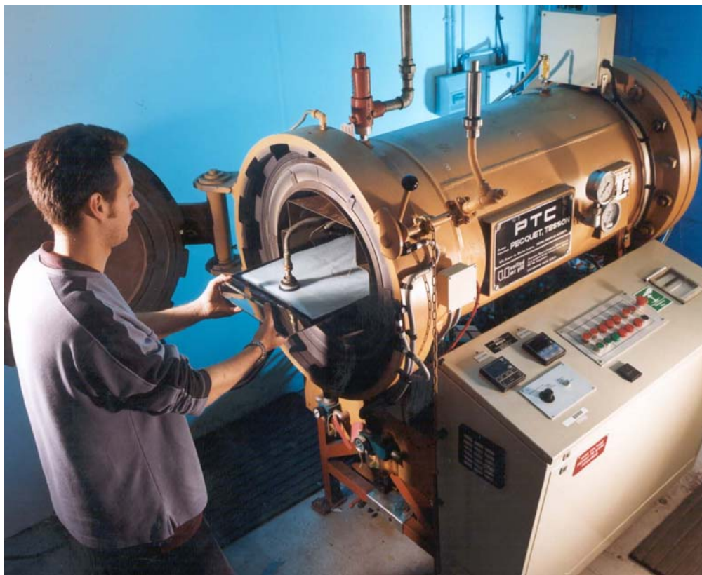
Figure 11: Temperature reference specimen manufacture in the NPL autoclave
