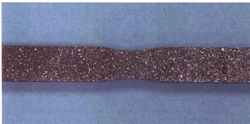
Figure 3 Specimen sprayed with speckle pattern
