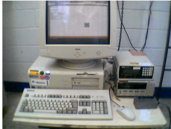
Figure 5. Apparatus used to measure continuity of daisy-chained components (PC controlled multiplexer and digital multimeter)
