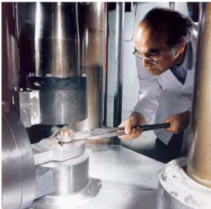
Figure 5. Hot billet being transferred from a furnace to the grabber arm on the Big Friction Rig.
