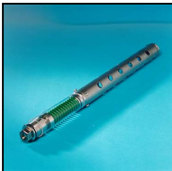
Figure 8 Self-loading tube for environmental stress cracking of plastics
