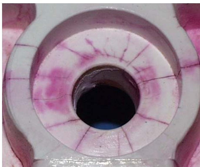
Figure 14 Red dye penetrant used to expose hairline cracking around bolthole in a plastic moulding
