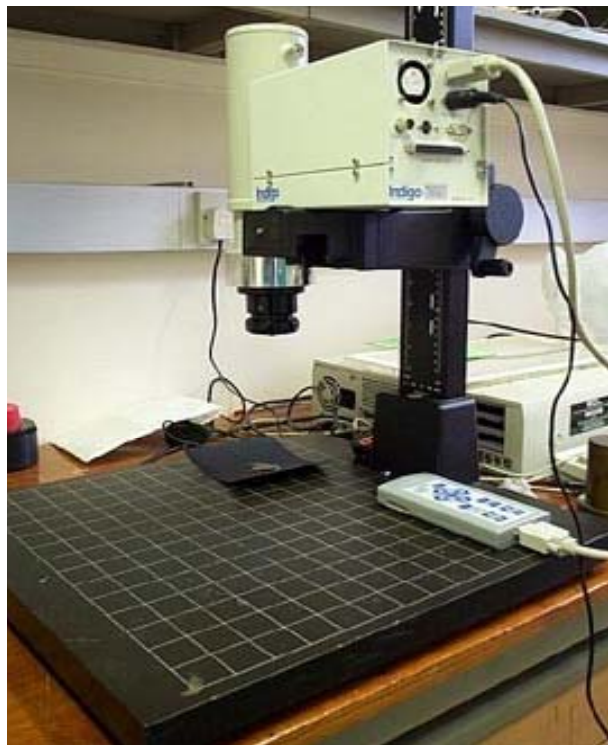
Figure 4.3 - Temperature measurement using 2-D infra-red camera.
