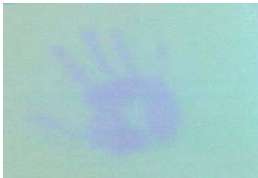
Figure 3.3 - Example of TLC operation: a hand in contact with the sheet shows a colour change compared to ambient.
