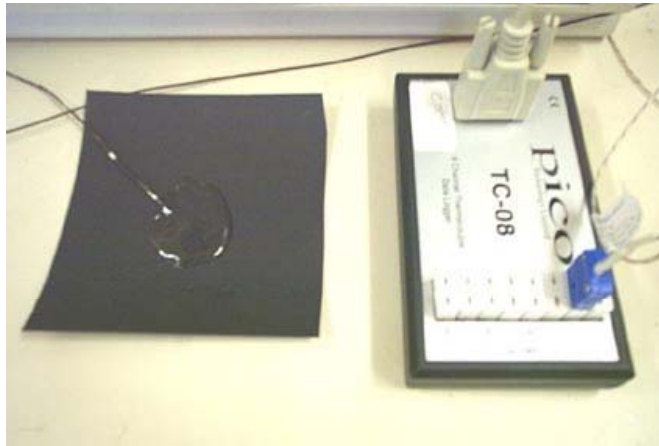
Figure 4.2 - Temperature measurement using T-type thermocouple and cold junction compensating data logger.
