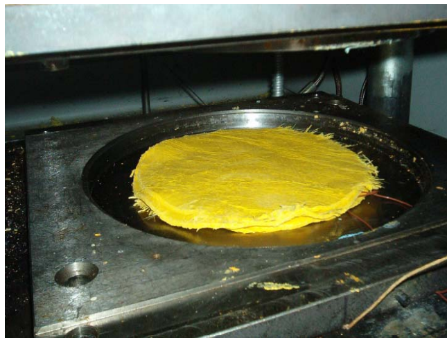
Figure 5.6 - Sensors positioned in material ‘charge’ inside modified pilot industrial tool.
