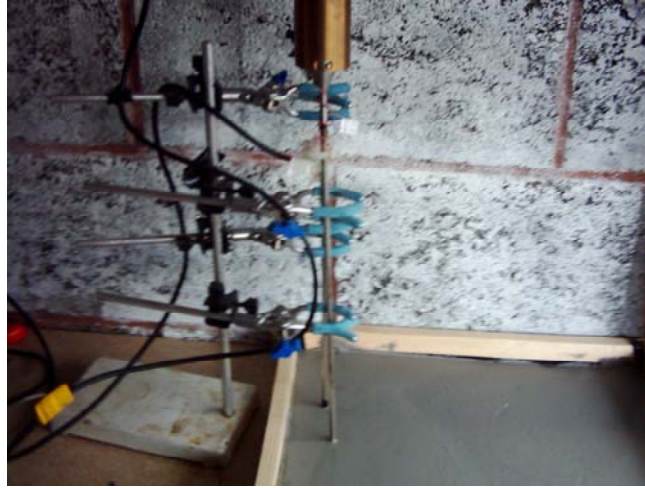
Figure 5.11 - Typical set-up for field trial acoustic cure monitoring measurements.
