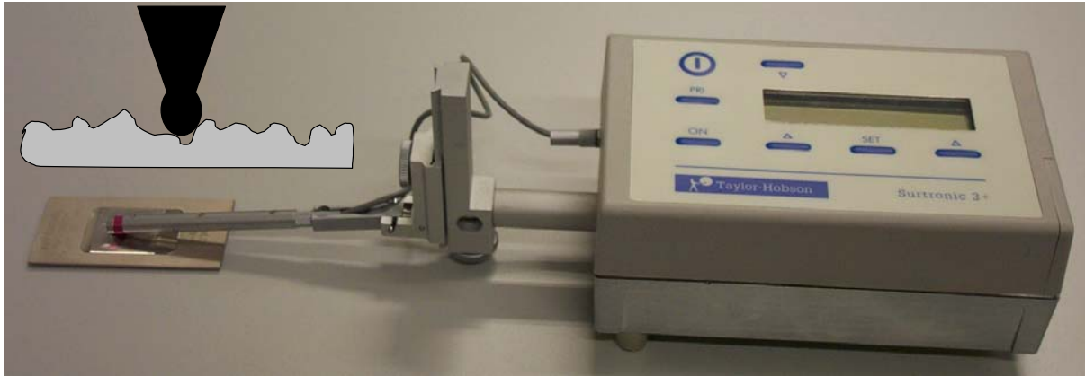
Figure 9: Contact (stylus) profilometry
