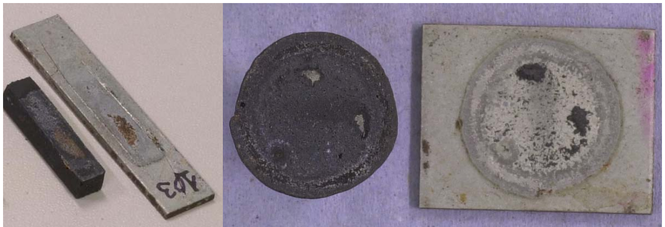
Figure 46: 3-point bend and pull-off samples tested after 44 days
